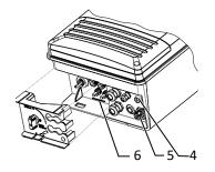
Fig. 16: Uncovering the DC connection
