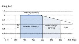
*Fig. 43:* Apparent power subject to grid voltage for devices below 12 kVA with UN 220/380, 230/400, 240/415V
