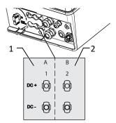
*Fig. 31:* Connection for DC positive and DC negative
