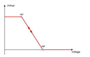
Fig. 48: Example characteristic curve without hysteresis
