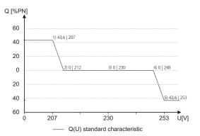
Fig. 44: Q(U) standard characteristic curve with 5 nodes
