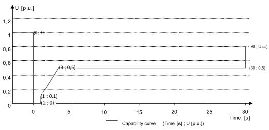
Fig. 56: Immunity to voltage dips characteristic curve relative to the nominal voltage
