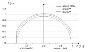
*Fig. 42:* P-Q operating range for devices below 12 kVA with  $U_N$  220/380, 230/400, 240/415V (Qmax=0.95Smax)
