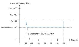
Fig. 45: Power gradient according to sample parameters and calculation
