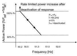
*Fig. 55:* P(f) example characteristic without hysteresis Mode 2
