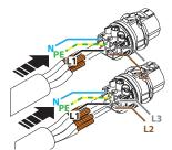
Fig. 20: Connect wires to the contact carrier
