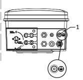
Fig. 32: Additional grounding point
