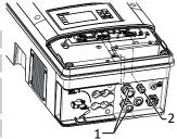
Fig. 34: Inserting the interface cable
