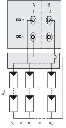
Fig. 28: Recommended standard connection *Fig. 29:* Parallel input with Y-adapter, short-circuits the unused MPP Tracker B
