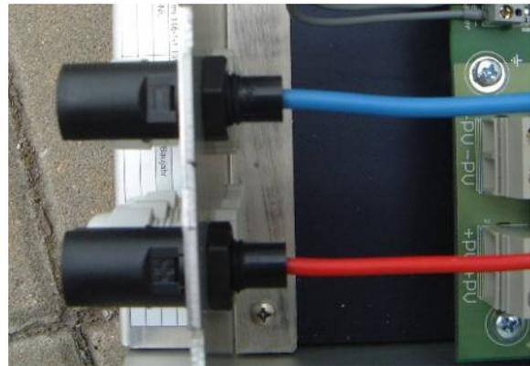
Figure 6.4: **Installing Tyco sockets**
