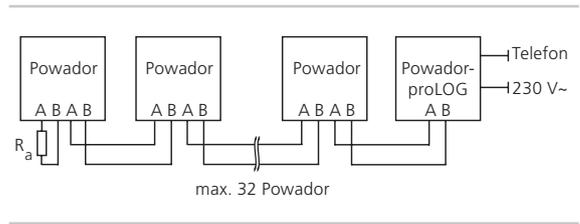
Figure 6.8: Connection diagram for the RS485 interface
