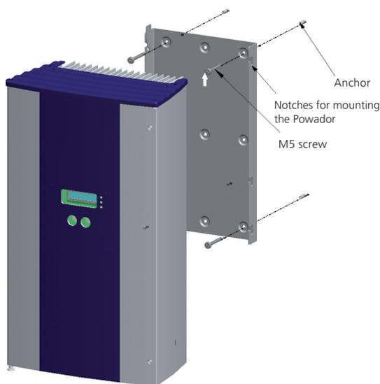
Figure 6.1: Powador wall bracket
