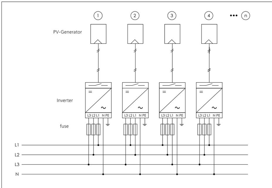
Figure 8.3: **Grid-side connection for installations with multiple inverters**
