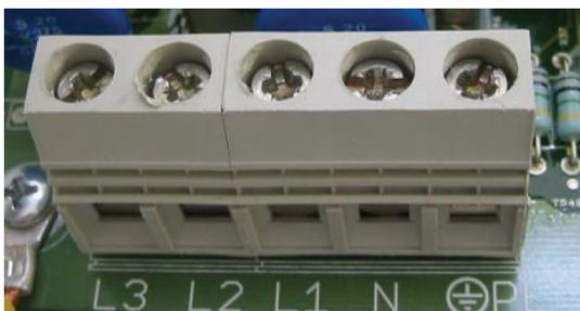
Figure 8.4: **Electrical connection**
