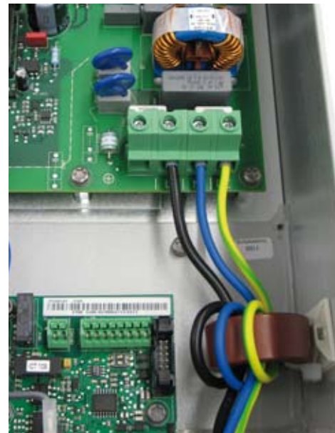
Figure 14: AC leads wound around the ferrite cores
