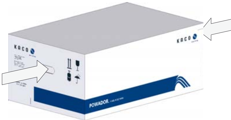
Figure 6: Transportation of the inverter
