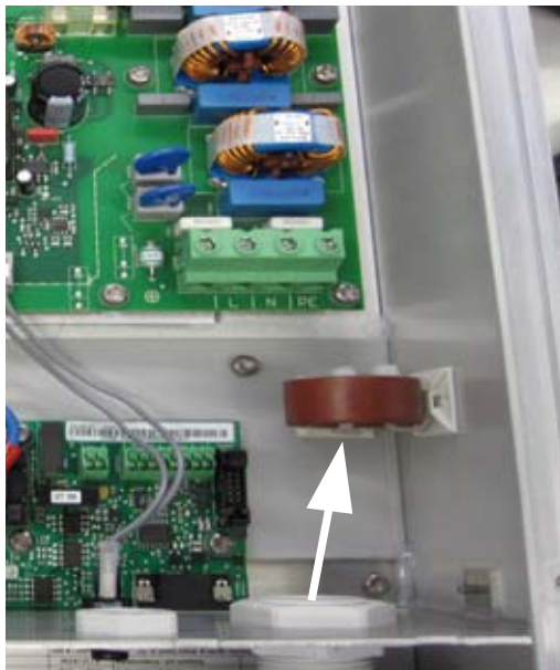
Figure 13: Insert AC leads into the connection area
